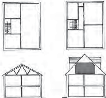
2.12 b Roof extensions.
